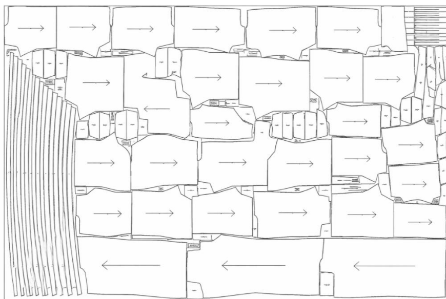
Figure 3. Marker Making for a Combination of 10 Sizes Garment
