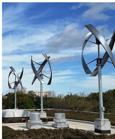
Figure 2. Vertical Axis Wind Turbine
