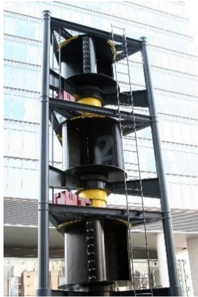
Figure 4. Savonius Wind Turbine
