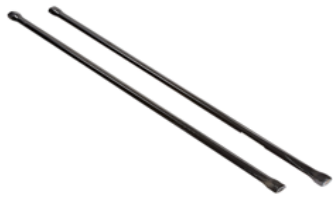
Figure 2. Existing Torsion Bar of Tank T-55
