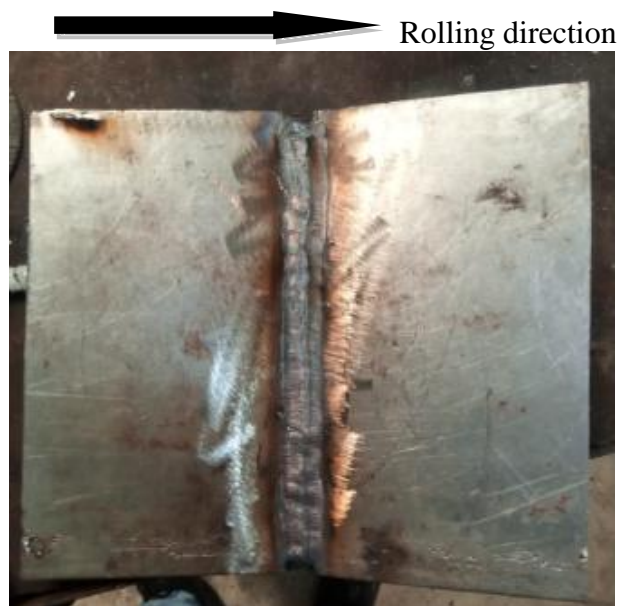
Figure 2: GTAW welded section of AISI 316L Austenitic stainless steel sample
