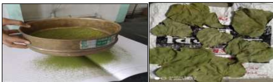
Figure 10. Dry Leaves and Powdered Leaves Passed Through Sieve
