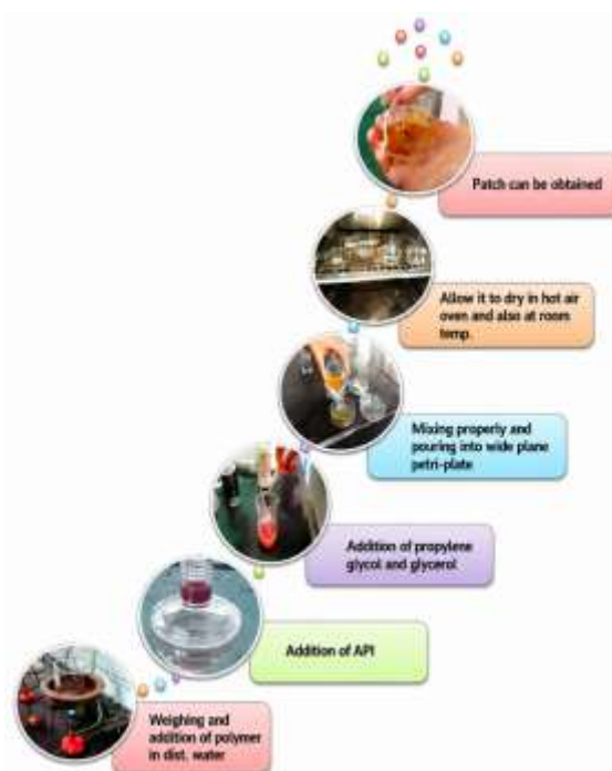
Figure 15. Stepwise Preparation of Polymeric Transdermal Patches by Solvent Casting Method
