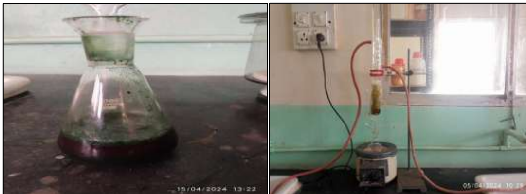
Figure 13. Extraction by Soxhlet Technique (Alcoholic) & Maceration (P.E.)
