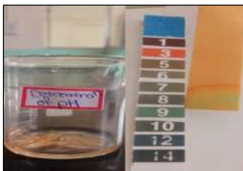
Figure 17. PH Paper Dipped Into Solution
