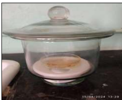
Figure 18. Desiccator Used to Remove Moisture
