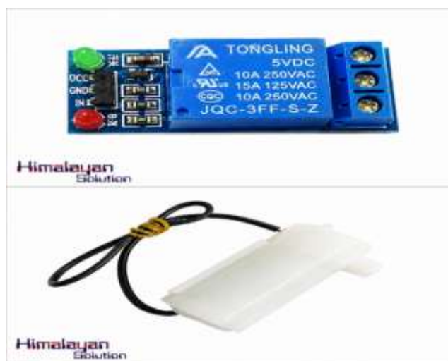
Figure 2. Water Pump with Relay
